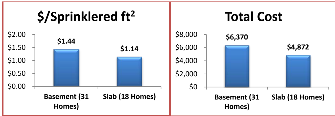
Figure 6. Sprinkler system cost by foundation type
